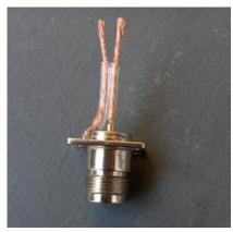
3. Solder a 1+ inch piece of speaker wire to the N connector. One wire goes to the center pin; the other wire to the outside part of the connector. I drilled a small hole in the connector flange for the wire to be inserted into and soldered in place. Leave about 3/4 inch of insulation on the speaker wire (as measured where the two wires are together). This is the transformer, transforming the antenna impedance to about 50 ohms.
