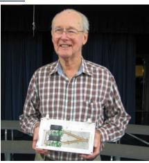
Herb Vanderbeek, WY6G, presented a coupler/attenuator with a heat sink and an amplifier (up to 140 W) for 1.2 GHz. Herb is showing the coupler in this photograph.
