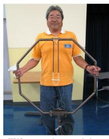
Toshi Sugiya, KJ6Q, presented a magnetic loop antenna with a capacitive trombone tuner, which he is showing here. The trombone tuner can quite plainly be seen. Toshi won the first place prize (a tie) for this entry.
